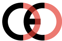
False CE Mark (too close)
